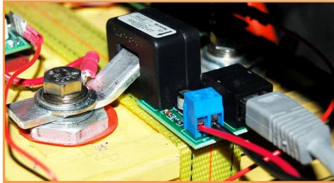
Constant Bluetooth communication between the sensor board hardware and the Android app allows real-time visualization of the selected EV parameters. When the EV is parked for charging in the garage, the Android device will allow remote monitoring of the charging state (Battery Remaining Charge Percentage gauge). The instructional installation video is available at: <http://www.youtube.com/watch?v=UkadxYN9EPw> and <http://youtu.be/H1xGzkuPNAw>
